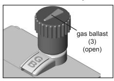
For **condensable vapors** (water vapor, solvents, etc.):
