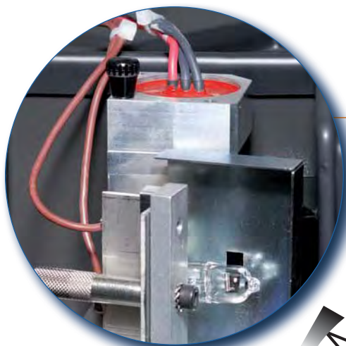
Lamps compartment thermally isolated from optical bench
