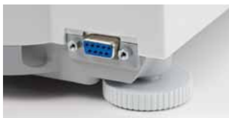
RS232 interface for data connectivity
