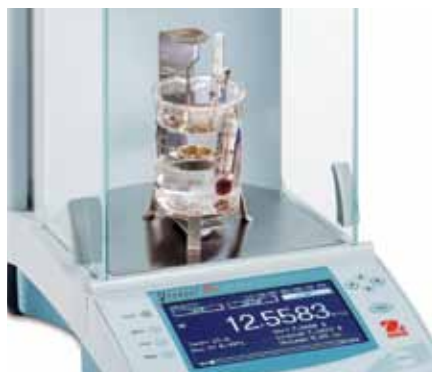
Voyager Pro shown with optional density determination kit.
