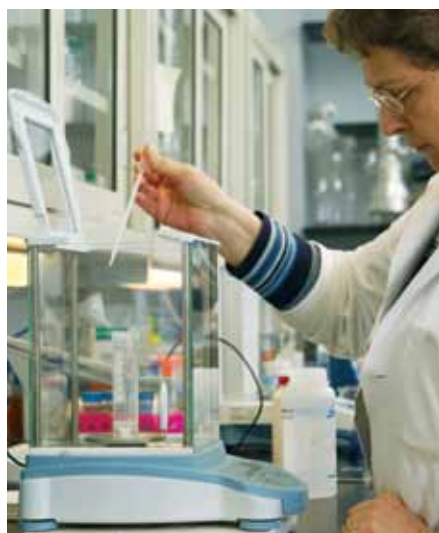
Removable front, side and back glass panels
