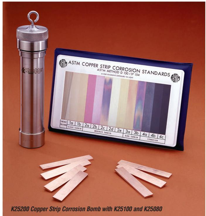
K25200 Copper Strip Corrosion Bomb with K25100 and K25080
