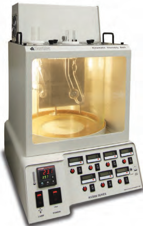
K23700 Constant Temperature Kinematic Viscosity Bath (KV3000)
