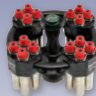
TX-100 Clinical Swinging Bucket Rotor with Carriers
