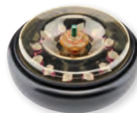
MT-12 Swinging Bucket Rotor
