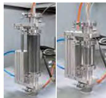
Thermocouple, type S with automatic pull-out device for precise control results in the low temperature range
