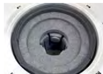
Graphite heating module
