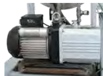
Vacuum pump for cold evacuation of the retort
