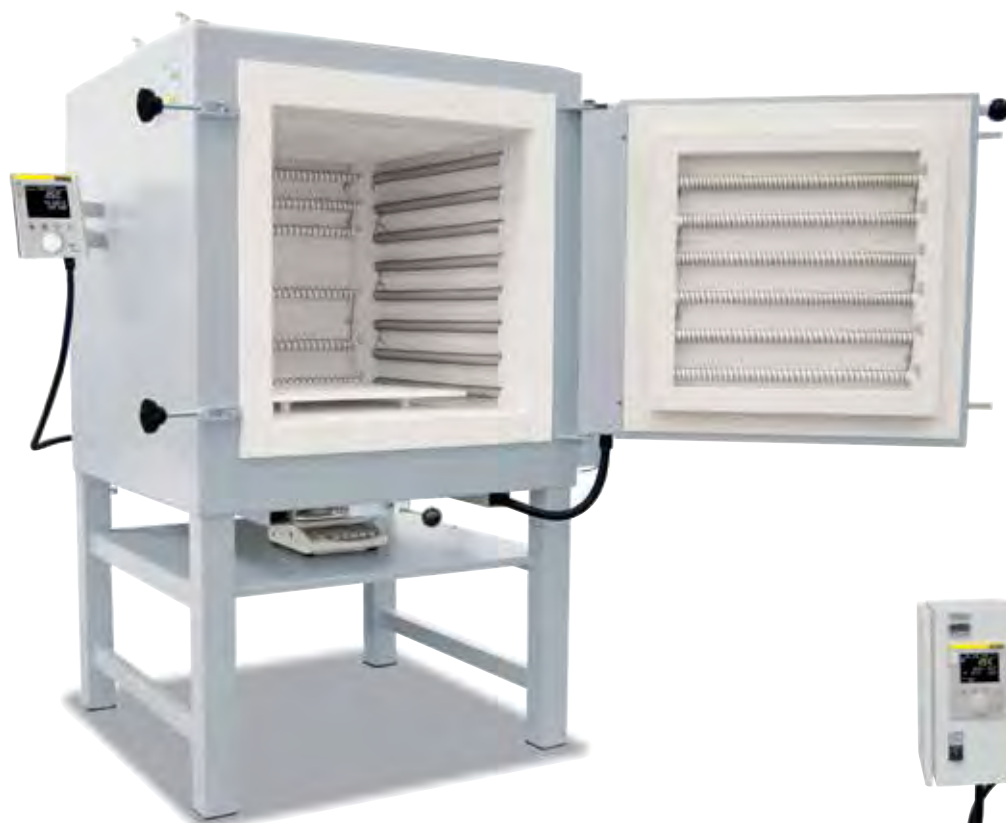
Chamber furnace LH 216/12SW with scale to measure weight reduction during annealing
