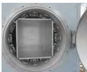
Inside heating in retort furnaces NRA ../06
