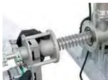
Screw-conveyor with adjustable speed
