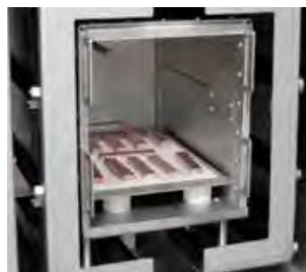
Heat treatment of copper bars under hydrogen in a retort furnace VHT 8/16-MO
