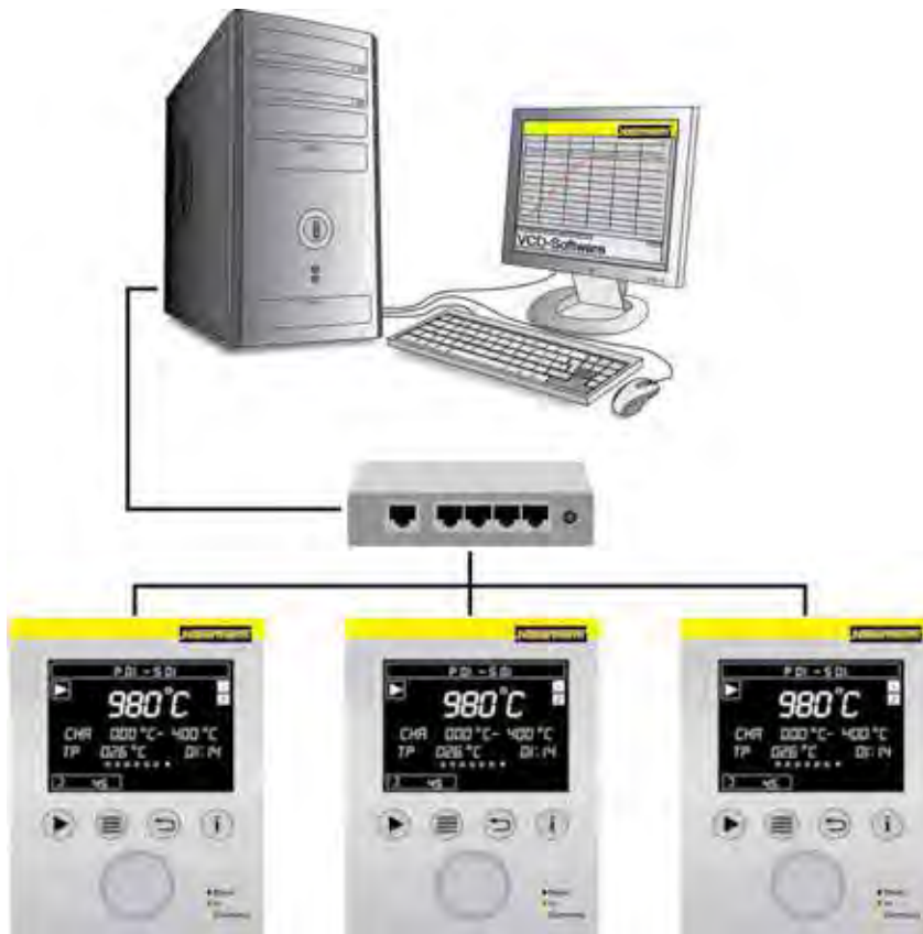
Example lay-out with 3 furnaces
