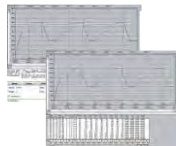
Software for documentation of the temperature curve and combustion loss using a PC
