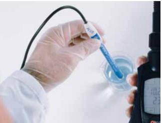
Special samples need special electrodes. SenTix® special electrodes can take on the challenges associated with measuring the pH value of surfaces, solids, suspensions, emulsions, low ionic samples, smallest volumes and more. For those who require a non-glass electrode: The
