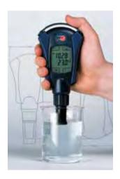
When the VARIO® is not being used for pH measurements, it can be used as a laboratory clock or timer.
